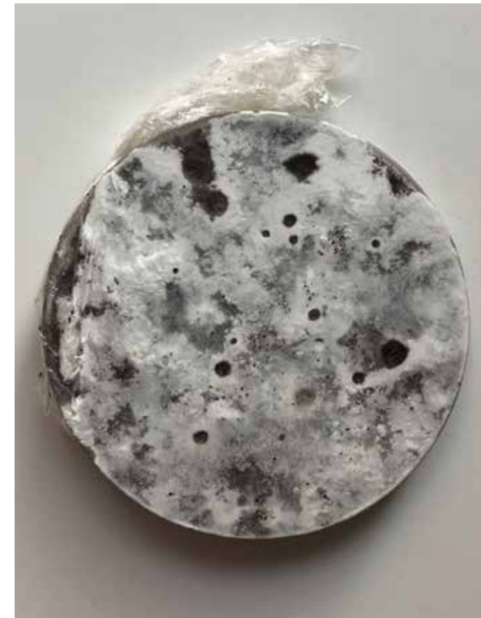
KAHVE ATIGINDAN YAPILAN MISELYUM MALZEME PETRİ KABINDA, 2021. FOTOĞRAF: DAMLA BURÇİN ATASOY MYCELIUM MATERIAL MADE FROM COFFEE WASTE IN PETRI BOWL, 2021. PHOTO: DAMLA BURÇİN ATASOY
